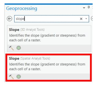
The Input Raster is Peavy DEM. Direct the output to McDonald.gdb and name it peavyslope. Change the Output measurement to Percent Rise - this will give us slope values as a percent rather than degrees. Click Run.
