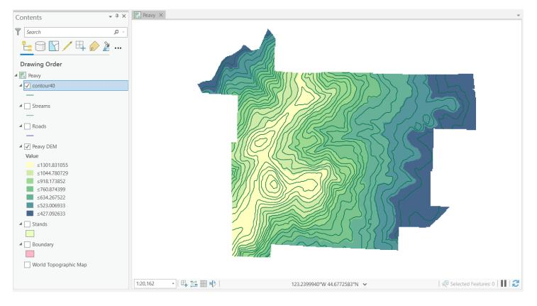
Open the attribute table for contour40 and notice that an elevation value (CONTOUR) was added to each row.
